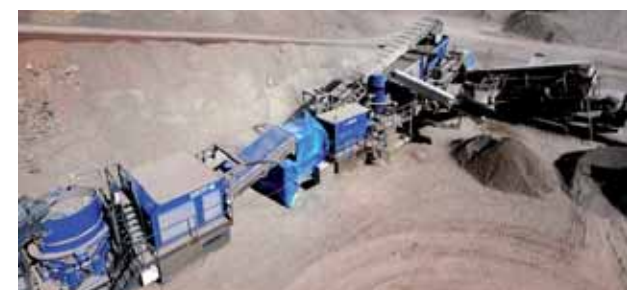
The MCO 11 S equipped with the KH 300 cone crusher forms part of a high-performance plant combination: one jaw crusher, two cone crushers and two screening plants supplied by Kleemann produce six high-quality end products in specified grain sizes.
