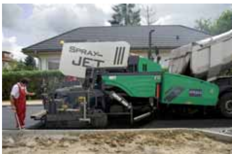
Compact, powerful and versatile: the SUPER 1800-2 can be used as a spray paver together with the SprayJet module or as a standard road paver.
