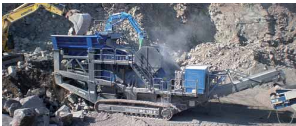
The MC 125 Z as part of a Kleemann plant combination operated in Scotland: the mobile jaw crusher was set up directly at the quarry face to pre-crush the 0 - 600 mm feed material to a 0 - 260 mm fraction.
