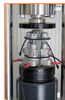
40x40x160mm cement prism fitted with three 55-C0222/F
