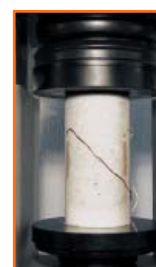
Determination of elastic modulus of cylindrical sample using surface mounted strain gauges.
