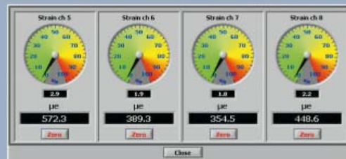
Virtual gauges indicating the actual reading of the sensor in percentage respect the full scale. It's an excellent tool for correct transducers positioning.
