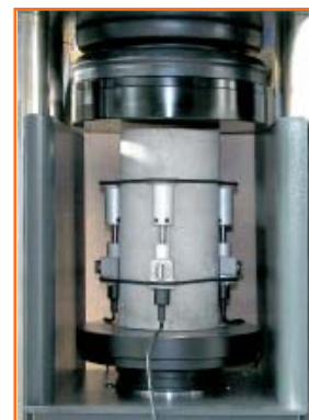
Three electronic compressometers 55-C0222/F fitted to a cylinder specimen during the compression stage.
