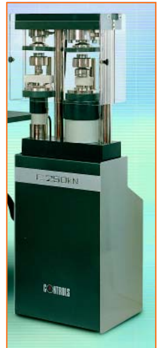
65-L1301/FR with fragment guard 65-L1300/P and flexural/compression devices available as accessory.
