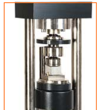
65-L1201/FR detail of round platen and load cell with compression device.
