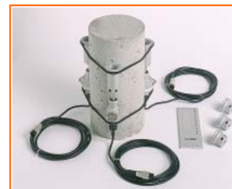
150 mm dia. x 300 mm cylindrical sample with 3 extension (compressometers 55-C0222/F ready for elastic modulus test).
