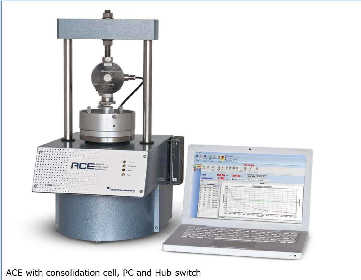
ACE with consolidation cell, PC and Hub-switch
