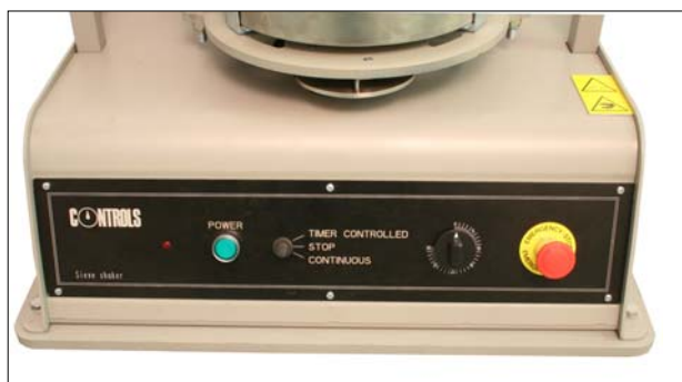
Front panel with mains switch and timer. Also shown is the optional base plate which is an alternative to floor fixing.
